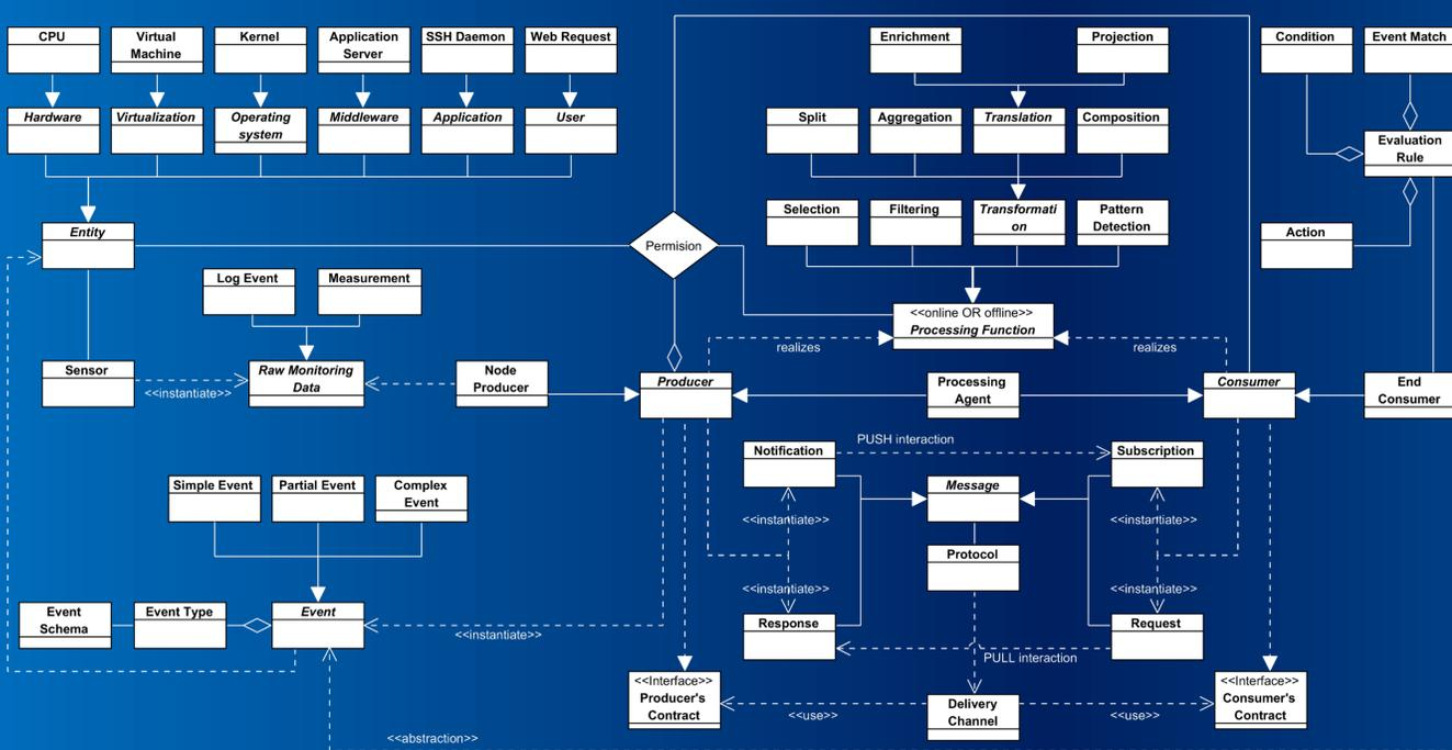
The model is founded on pattern-based publish-subscribe interaction and Complex Event Processing principles [3] with support for multi-tenancy. The monitored entities can belong to any of the main cloud layers.
